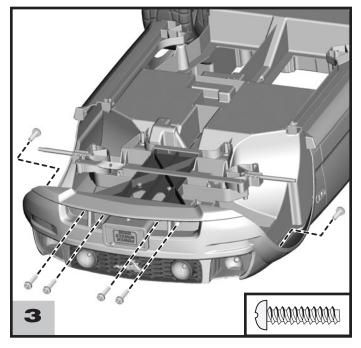
• Insert six #8 x  $^{3}/_{4}$ " screws into the front bumper and tighten.
